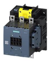
power contactor, AC-3e/AC-3 185 A, 90 kW / 400 V AC (50-60 Hz) / DC Uc: 96-127 V x (0.8-1.1) F-PLC input 24 V DC 3-pole, auxiliary contacts 2 NO + 2 NC drive: electronic main circuit: busbar control and auxiliary circuit: screw terminal
