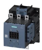
power contactor, AC-3e/AC-3 185 A, 90 kW / 400 V AC (50-60 Hz) / DC Uc: 220-240 V 3-pole, auxiliary contacts 2 NO + 2 NC solid-state compatible drive: conventional main circuit: busbar control and auxiliary circuit: screw terminal
