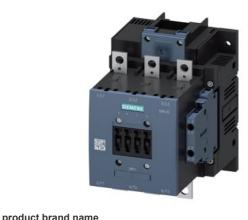
contactor, 100HP, 460 / 575 V AC (50...60 Hz) / DC operation 220 ... 240 V AC/DC auxiliary contacts 2 NO + 2 NC 3-pole, frame size S6 busbar connections drive: conventional NEMA size 4
