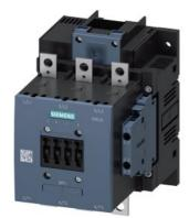
power contactor, AC-3e/AC-3 185 A, 90 kW / 400 V AC (50-60 Hz) / DC Uc: 23-26 V 3-pole, auxiliary contacts 2 NO + 2 NC drive: conventional main circuit: busbar control and auxiliary circuit: screw terminal
