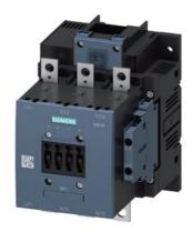
power contactor, AC-3e/AC-3 185 A, 90 kW / 400 V AC (50-60 Hz) / DC Uc: 23-26 V 3-pole, auxiliary contacts 2 NO + 2 NC drive: conventional main circuit: busbar control and auxiliary circuit: screw terminal reusable packaging = 9 units
