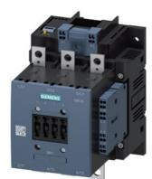
power contactor, AC-3e/AC-3 185 A, 90 kW / 400 V Uc: 24 V DC x (0.7-1.25) PLC input 24-110 V DC 3-pole, auxiliary contacts 2 NO + 2 NC drive: electronic main circuit: busbar control and auxiliary circuit: spring-loaded terminal extended rated condition railroad IEC 60077
