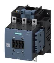
power contactor, AC-3e/AC-3 185 A, 90 kW / 400 V AC (50-60 Hz) / DC Uc: 96-127 V PLC input 24 V DC 3-pole, auxiliary contacts 2 NO + 2 NC drive: electronic main circuit: busbar control and auxiliary circuit: spring-loaded terminal
