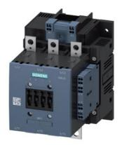
power contactor, AC-3e/AC-3 185 A, 90 kW / 400 V AC (50-60 Hz) / DC Uc: 220-240 V 3-pole, auxiliary contacts 2 NO + 2 NC drive: conventional main circuit: busbar control and auxiliary circuit: spring-loaded terminal
