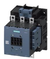
power contactor, AC-3e/AC-3 185 A, 90 kW / 400 V AC (50-60 Hz) / DC Uc: 110-127 V 3-pole, auxiliary contacts 2 NO + 2 NC drive: conventional main circuit: busbar control and auxiliary circuit: spring-loaded terminal
