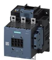
power contactor, AC-3e/AC-3 150 A, 75 kW / 400 V Uc: 24 V DC x (0.7-1.25) PLC input 24-110 V DC 3-pole, auxiliary contacts 2 NO + 2 NC drive: electronic main circuit: busbar control and auxiliary circuit: screw terminal extended rated condition railroad IEC 60077
