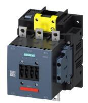
power contactor, AC-3e/AC-3 150 A, 75 kW / 400 V AC (50-60 Hz) / DC Uc: 200-277 V x (0.8-1.1) F-PLC input 24 V DC 3-pole, auxiliary contacts 2 NO + 2 NC permanently mounted drive: electronic main circuit: busbar control and auxiliary circuit: screw terminal
