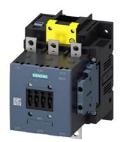
power contactor, AC-3e/AC-3 150 A, 75 kW / 400 V AC (50-60 Hz) / DC Uc: 96-127 V x (0.8-1.1) F-PLC input 24 V DC 3-pole, auxiliary contacts 2 NO + 2 NC drive: electronic main circuit: busbar control and auxiliary circuit: screw terminal
