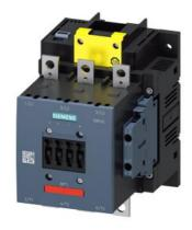
power contactor, AC-3e/AC-3 150 A, 75 kW / 400 V AC (50-60 Hz) / DC Uc: 96-127 V x (0.8-1.1) F-PLC input 24 V DC 3-pole, auxiliary contacts 2 NO + 2 NC permanently mounted drive: electronic main circuit: busbar control and auxiliary circuit: screw terminal
