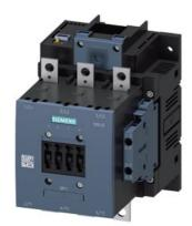
power contactor, AC-3e/AC-3 150 A, 75 kW / 400 V AC (50-60 Hz) / DC Uc: 96-127 V PLC input 24 V DC 3-pole, auxiliary contacts 2 NO + 2 NC drive: electronic main circuit: busbar control and auxiliary circuit: screw terminal
