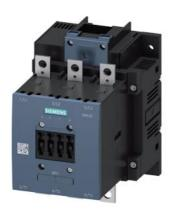
power contactor, AC-3e/AC-3 150 A, 75 kW / 400 V AC (50-60 Hz) / DC Uc: 220-240 V 3-pole, without auxiliary contacts drive: conventional main circuit: busbar control and auxiliary circuit: screw terminal
