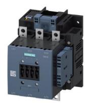
power contactor, AC-3e/AC-3 150 A, 75 kW / 400 V AC (50-60 Hz) / DC Uc: 200-277 V PLC input 24 V DC 3-pole, auxiliary contacts 2 NO + 2 NC drive: electronic main circuit: busbar control and auxiliary circuit: spring-loaded terminal
