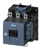
power contactor, AC-3e/AC-3 150 A, 75 kW / 400 V AC (50-60 Hz) / DC Uc: 110-127 V 3-pole, auxiliary contacts 2 NO + 2 NC drive: conventional main circuit: busbar control and auxiliary circuit: spring-loaded terminal
