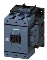
power contactor, AC-3e/AC-3 115 A, 55 kW / 400 V, AC (50-60 Hz) / DC Uc: 440-480 V 3-pole, auxiliary switch right 3RH1921-2DE11 drive: conventional main circuit: box terminal control and auxiliary circuit: screw terminal
