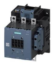
power contactor, AC-3e/AC-3 115 A, 55 kW / 400 V, Uc: 24 V DC x (0.7-1.25) PLC input 24-110 V DC 3-pole, auxiliary contacts 2 NO + 2 NC drive: electronic main circuit: busbar control and auxiliary circuit: screw terminal
