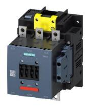
power contactor, AC-3e/AC-3 115 A, 55 kW / 400 V, AC (50-60 Hz) / DC Uc: 200-277 V x (0.8-1.1) F-PLC input 24 V DC 3-pole, auxiliary contacts 2 NO + 2 NC permanently mounted drive: electronic main circuit: busbar control and auxiliary circuit: screw terminal
