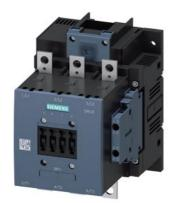
power contactor, AC-3e/AC-3 115 A, 55 kW / 400 V, AC (50-60 Hz) / DC Uc: 575-600 V 3-pole, auxiliary contacts 2 NO + 2 NC drive: conventional main circuit: busbar control and auxiliary circuit: screw terminal
