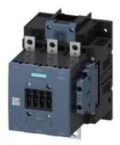
power contactor, AC-3e/AC-3 115 A, 55 kW / 400 V, AC (50-60 Hz) / DC Uc: 220-240 V 3-pole, auxiliary contacts 2 NO + 2 NC drive: conventional main circuit: busbar control and auxiliary circuit: screw terminal
