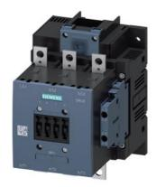
power contactor, AC-3e/AC-3 115 A, 55 kW / 400 V, AC (50-60 Hz) / DC Uc: 110-127 V 3-pole, auxiliary contacts 2 NO + 2 NC drive: conventional main circuit: busbar control and auxiliary circuit: screw terminal
