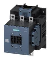
power contactor, AC-3e/AC-3 115 A, 55 kW / 400 V, AC (50-60 Hz) / DC Uc: 23-26 V 3-pole, auxiliary contacts 2 NO + 2 NC drive: conventional main circuit: busbar control and auxiliary circuit: screw terminal
