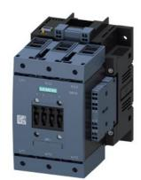
power contactor, AC-3e/AC-3 115 A, 55 kW / 400 V, Uc: 24 V DC x (0.7-1.25) PLC input 24-110 V DC 3-pole, auxiliary contacts 2 NO + 2 NC drive: electronic main circuit: box terminal control and auxiliary circuit: spring-loaded terminal
