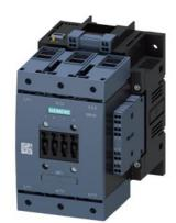
power contactor, AC-3e/AC-3 115 A, 55 kW / 400 V, AC (50-60 Hz) / DC Uc: 21-27.3 V PLC input 24 V DC 3-pole, auxiliary contacts 2 NO + 2 NC drive: electronic main circuit: box terminal control and auxiliary circuit: spring-loaded terminal
