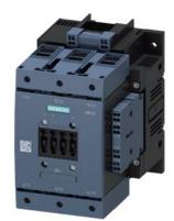
power contactor, AC-3e/AC-3 115 A, 55 kW / 400 V, AC (50-60 Hz) / DC Uc: 220-240 V 3-pole, auxiliary contacts 2 NO + 2 NC drive: conventional main circuit: box terminal control and auxiliary circuit: spring-loaded terminal
