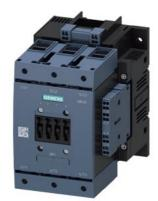
power contactor, AC-3e/AC-3 115 A, 55 kW / 400 V, AC (50-60 Hz) / DC Uc: 23-26 V 3-pole, auxiliary contacts 2 NO + 2 NC drive: conventional main circuit: box terminal control and auxiliary circuit: spring-loaded terminal
