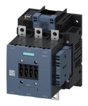
power contactor, AC-3e/AC-3 115 A, 55 kW / 400 V, AC (50-60 Hz) / DC Uc: 200-277 V PLC input 24 V DC 3-pole, auxiliary contacts 2 NO + 2 NC drive: electronic main circuit: busbar control and auxiliary circuit: spring-loaded terminal
