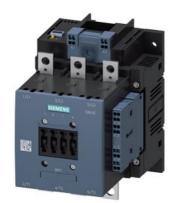
power contactor, AC-3e/AC-3 115 A, 55 kW / 400 V, AC (50-60 Hz) / DC Uc: 96-127 V PLC input 24 V DC 3-pole, auxiliary contacts 2 NO + 2 NC drive: electronic main circuit: busbar control and auxiliary circuit: spring-loaded terminal
