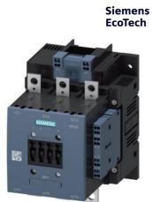
power contactor, AC-3e/AC-3 115 A, 55 kW / 400 V, AC (50-60 Hz) / DC Uc: 220-240 V 3-pole, auxiliary contacts 2 NO + 2 NC drive: conventional main circuit: busbar control and auxiliary circuit: spring-loaded terminal
