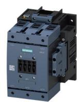
power contactor, AC-3e/AC-3 115 A, 55 kW / 400 V, AC (50-60 Hz) / DC Uc: 21-27.3 V PLC input 24 V DC 3-pole, auxiliary contacts 2 NO + 2 NC drive: electronic main circuit: box terminal control and auxiliary circuit: screw terminal
