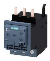
Monitoring relay, can be mounted to Contactor 3RT2, Size S2 basic, analog adjustment Apparent current monitoring 8...80 A, 50...60 Hz, 2-phase Supply 24 V AC/DC 1 change-over contact Monitoring for Current overshoot and undershoot Phase failure, Cable break with or without fault buffer ON delay 0-60 s Noise pulse suppression 0-30 s Switching hysteresis 6% spring-type connection system
