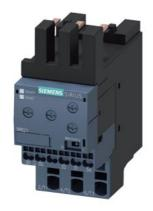
Monitoring relay, can be mounted to Contactor 3RT2, Size S0 basic, analog adjustment Apparent current monitoring 4...40 A, 50...60 Hz, 2-phase Supply 24 V AC/DC 1 change-over contact Monitoring for Current overshoot and undershoot Phase failure, Cable break with or without fault buffer ON delay 0-60 s Noise pulse suppression 0-30 s Switching hysteresis 6% spring-type connection system
