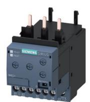
Monitoring relay, can be mounted to Contactor 3RT2, Size S0 basic, analog adjustment Apparent current monitoring 4...40 A, 50...60 Hz, 2-phase Supply 24-240 V AC/DC 1 change-over contact Monitoring for Current overshoot and undershoot Phase failure, Cable break with or without fault buffer ON delay 0-60 s Noise pulse suppression 0-30 s Switching hysteresis 6% Screw connection system
