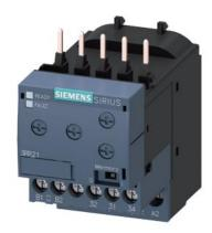
Monitoring relay, can be mounted to Contactor 3RT2, Size S00 basic, analog adjustment Apparent current monitoring 1.6-16 A, 20-400 Hz, 2-phase Supply 24-240 V AC/DC 1 change-over contact Monitoring for Current overshoot and undershoot Phase failure, Cable break with or without fault buffer ON delay 0-60 s Noise pulse suppression 0-30 s Switching hysteresis 6% Screw connection system
