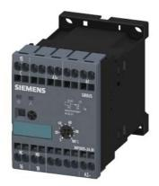
Timing relay, electronic slow-operating 1 change-over contact 24 V AC/DC, 200 to 240 V AC at 50/60~Hz AC 0.05~s to 100~h Overall width 45~mm Spring-type terminal
