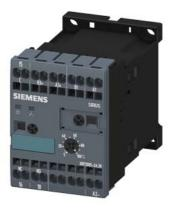
Timing relay, electronic Multifunction, 8 functions 1 change-over contact 24 V AC/DC, 200 to 240 V AC at 50/60 Hz AC 0.05 s to 100 h Overall width 45 mm Spring-type terminal
