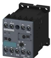
Timing relay, electronic Multifunction, 16 functions 2 change-over contacts 24 to 240 V AC/DC at 50/60 Hz AC 0.05 s to 100 h Overall width 45 mm screw terminal
