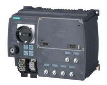
SIRIUS motor starter M200D Technology module Reversing starter Electronic switching AC-3, 5.5 kW / 400 V 1.5 A...12.00 A Electronic overload protection Thermistor: THERMOCLICK / PTC without brake contact 4 DI / 2 DO Han Q4/2 - Han Q8/0 with manual on-site operation and key-operated switch via communication module 3RK1305\* can be used on PROFIBUS or PROFINET
