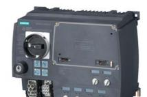
SIRIUS motor starter M200D technology module direct-on-line starter electronic switching AC-3, 5.5 kW / 400 V 1.5 A...12.00 A electronic overload protection thermistor: thermoclick / PTC without brake contact 4 DI / 2 DO Han Q4/2 - Han Q8/0 with manual on-site operation and keyswitch via communications module 3RK1305\* can be used on PROFIBUS or PROFINET
