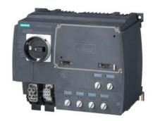
SIRIUS motor starter M200D technology module direct-on-line starter electronic switching AC-3, 5.5 kW / 400 V 1.5 A...12.00 A electronic overload protection thermistor: thermoclick / PTC without brake contact 4 DI / 2 DO Han Q4/2 - Han Q8/0 via communications module 3RK1305\* can be used on PROFIBUS or PROFINET
