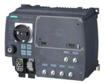
SIRIUS motor starter M200D technology module reversing starter mechanical switching AC-3, 5.5 kW / 400 V 1.5 A...12.00 A electronic overload protection thermistor: thermoclick / PTC without brake contact 4 DI / 2 DO Han Q4/2 - Han Q8/0 with manual on-site operation and keyswitch via communications module 3RK1305\* can be used on PROFIBUS or PROFINET
