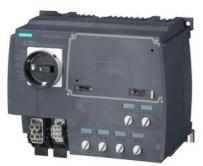
SIRIUS motor starter M200D Technology module Reversing starter Mechanical switching AC-3, 5.5 kW / 400 V 1.5 A...12.00 A Electronic overload protection Thermistor: THERMOCLICK / PTC without brake contact 4 DI / 2 DO Han Q4/2 - Han Q8/0 via communication module 3RK1305\* can be used on PROFIBUS or PROFINET
