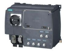
SIRIUS motor starter M200D Technology module DOL starter Mechanical switching AC-3, 5.5 kW / 400 V 1.5 A...12.00 A Electronic overload protection Thermistor: THERMOCLICK / PTC with brake contact 180 V DC 4 DI / 2 DO Han Q4/2 - Han Q8/0 via communication module 3RK1305\* can be used on PROFIBUS or PROFINET
