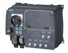
SIRIUS motor starter M200D Technology module Reversing starter Electronic switching AC-3, 0.75KW / 400 V 0.15 A...2.00 A Electronic overload protection Thermistor: THERMOCLICK / PTC without brake contact 4 DI / 2 DO Han Q4/2 - Han Q8/0 with manual on-site operation and key-operated switch via communication module 3RK1305\* can be used on PROFIBUS or PROFINET
