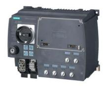
SIRIUS motor starter M200D Technology module DOL starter Electronic switching AC-3, 0.75KW / 400 V 0.15 A...2.00 A Electronic overload protection Thermistor: THERMOCLICK / PTC with brake contact 180 V DC 4 DI / 2 DO Han Q4/2 - Han Q8/0 with manual on-site operation and key-operated switch via communication module 3RK1305\* can be used on PROFIBUS or PROFINET
