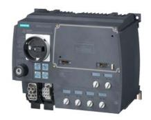
SIRIUS motor starter M200D technology module direct-on-line starter electronic switching AC-3, 0.75 kW/400 V 0.15 A...2.00 A electronic overload protection thermistor: thermoclick / PTC without brake contact 4 DI / 2 DO Han Q4/2 - Han Q8/0 with manual on-site operation and keyswitch via communications module 3RK1305\* can be used on PROFIBUS or PROFINET
