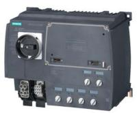
SIRIUS motor starter M200D Technology module DOL starter Electronic switching AC-3, 0.75KW / 400 V 0.15 A...2.00 A Electronic overload protection Thermistor: THERMOCLICK / PTC without brake contact 4 DI / 2 DO Han Q4/2 - Han Q8/0 via communication module 3RK1305\* can be used on PROFIBUS or PROFINET
