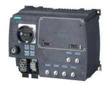
SIRIUS motor starter M200D Technology module Reversing starter Mechanical switching AC-3, 0.75KW / 400 V 0.15 A...2.00 A Electronic overload protection Thermistor: THERMOCLICK / PTC without brake contact 4 DI / 2 DO Han Q4/2 - Han Q8/0 with manual on-site operation and key-operated switch via communication module 3RK1305\* can be used on PROFIBUS or PROFINET
